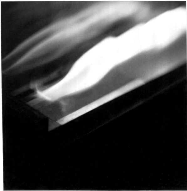
Fig. 8 Bird's eye view of separated flame for rectangular cylinder ( D = 10\text{ mm} , H = 10\text{ mm} , U_\infty = 1.5\text{ m/s} , and v_w = 0.07\text{ m/s} ).
