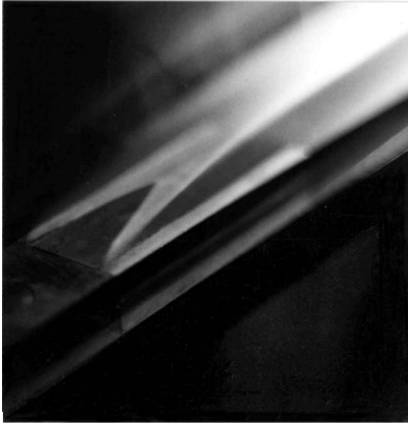
Fig. 6 Bird's eye view of symmetric separated flame for no obstacle ( U_\infty = 1.5 m/s and v_w = 0.07 m/s).
